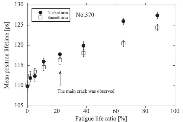
Fig.9 The mean positron lifetime of No.370.
