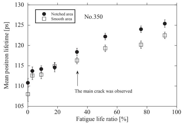
Fig.8 The mean positron lifetime of No.350.
