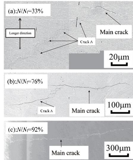
Fig.7 Results of SEM observation of No.350.
